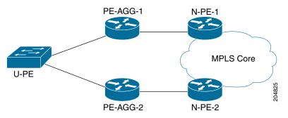
The first topology (N-PE redundancy starting at the U-PE, as shown in Figure D-1) provides the model of fault recovery for the N-PE device. As shown in the diagram, there are two different outgoing interfaces starting from the U-PE device. Each terminates at a different N-PE.
